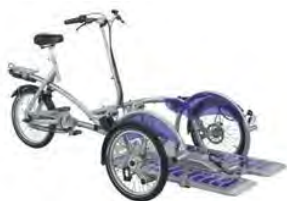
Wheelchair transporter (Van Raam 2012) for wheelchairs up to 74 cms width plus passenger.
